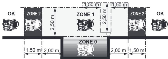
Install the pump in a dry, well-ventilated place. The motor requires the air to circulate freely around it to allow natural ventilation. Check regularly that no objects, leaves or other debris are blocking the motor cooling system.
